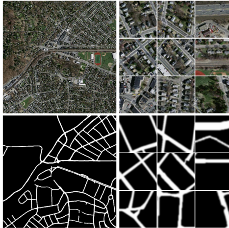
Figure 2: Remote sensing road dataset. This dataset is characterized by low resolution of small targets. In the image, the maximum road width is 30 pixels, and the minimum is less than 5 pixels.
